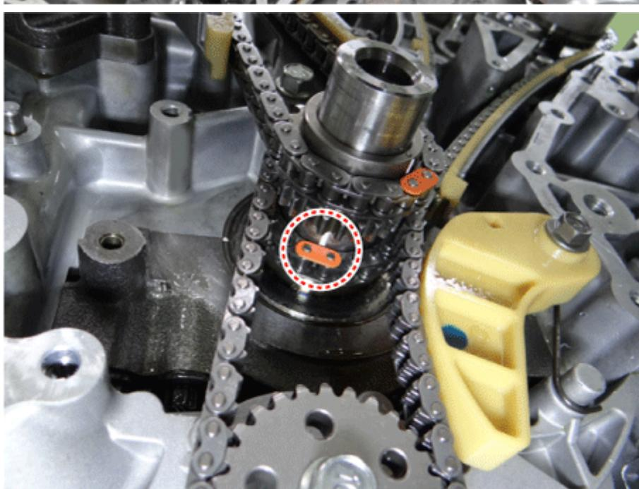
4. Release the ratchet by pulling the link down using a thin rod. Compress the piston and then insert a stopper into the hole on the ratchet to hold the compressed piston.
